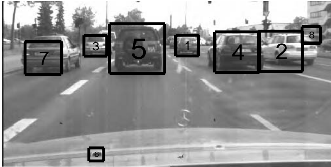
Fig. 4. Vehicle component-based spatio-temporal object detection for multiple targets. The algorithm was queried for 8 targets. The mean of 30 samples from the belief for each object are shown in red. Targets are found one at the time using an iterative approach that adjusts the likelihood functions to down weight regions where targets have already been found.
