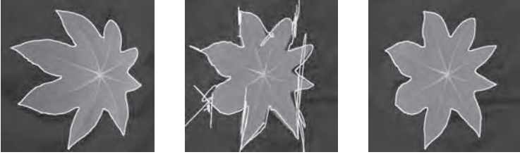
Fig. 1. Demonstration of filter accuracy by optical flow tracking. Left: first image. Middle: tracked with 3-tab derivative. Right: tracked with 5-tab optimized filter family.
