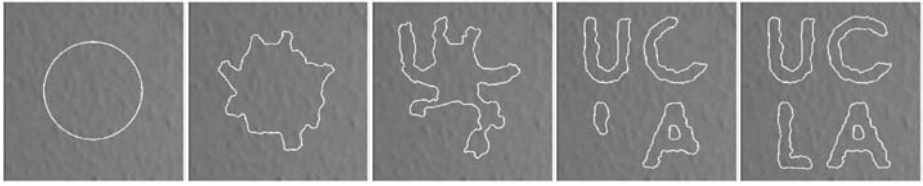
Fig. 2. Accurate motion segmentation. Contour evolution obtained with functional (26) and parameter values \nu = 0.06 , \sigma = 1 , superimposed on one of the two input frames. The input images show the text region (Figure 1, right side) of the wallpaper moving to the right and the remainder moving to the left. The motion competition framework generates highly accurate segmentations, even if the input images exhibit little in terms of salient features. Due to the region-based formulation, the initial contour does not need to be close to the final segmentation. We found that alternative initializations generate essentially identical segmentation results. The contour evolution took approximately 10 seconds in Matlab.
